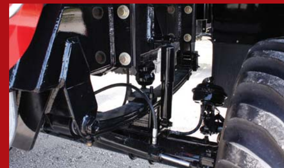
Heavy Duty double-reduction Axletech rear axle
