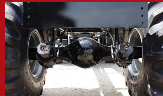
Heavy Duty double-reduction Axletech rear axle
