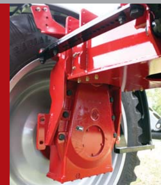
Heavy duty cast iron all-gear drop boxes
