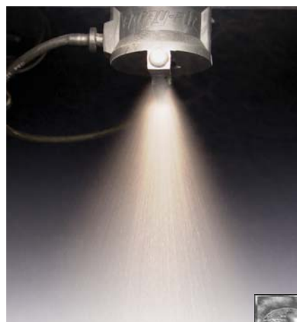
Droplet size set at 100/120 microns.
