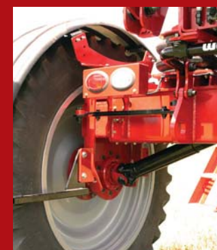
Welded box style leg construction with angle drive shafts
