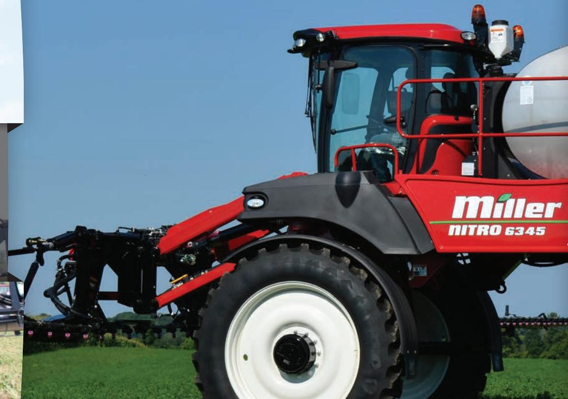
With the 4-wheel steer option, you'll have the tightest turning radius in the business. With front and rear wheels following the same track, crop damage is minimized and headland turning is a snap.
